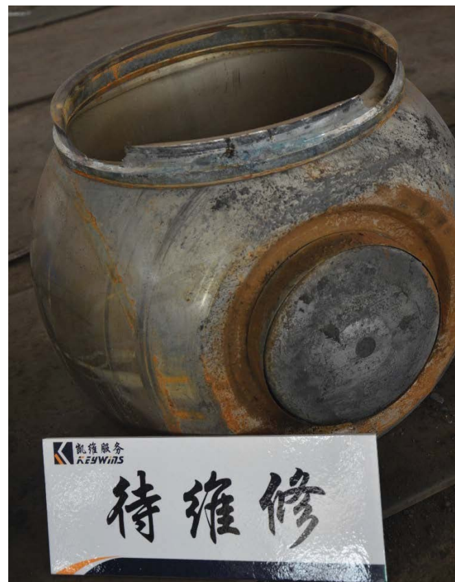
阀座严重冲蚀
