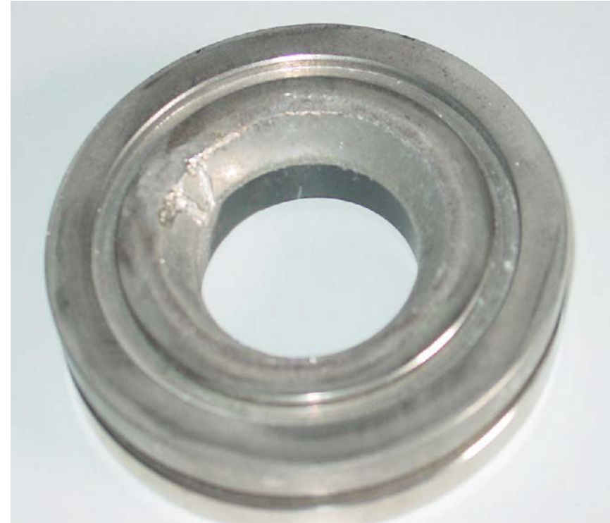
Worn out Valve Seat Removed from a high-pressure slurry pump
